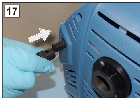
17. Place the cap on the gas ballast.
