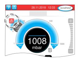
Warnings and / or errors are indicated by a flashing pressure curve. If the flashing pressure curve is pressed, the process with fault can be called up. The process without fault continues operation. If both processes are affected by the fault, both processes stop.
