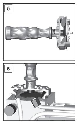
5. Lift the diaphragm at the side. Place the diaphragm carefully together with the diaphragm clamping disc and the diaphragm support disc in the diaphragm key. Avoid damage of the dia-
