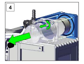
Loosen the four Allen head screws; Allen key size 5. Remove the catchpot. Pay attention to the sealing ring.
