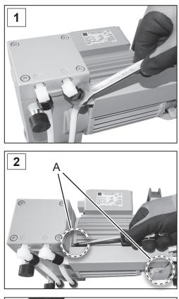
Loosen the union nuts at the pump heads; open-ended wrench width 17 mm.
