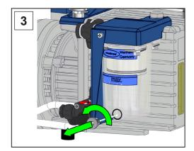
**3.** Open the drain screw of the transparent catchpot and drain the condensate; Allen key size 6. Pay attention to the O-ring.
