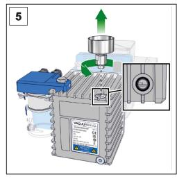
Unscrew the manometer at its adapter from the oil reservoir of the rotary vane pump; open-ended wrench width 17 mm. Do not turn the manometer itself as leaks might be caused! Pay attention to the O-ring.
