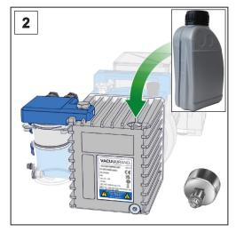
Pour only approx. 350 ml (0.37 quarts) of pump oil into the pump, bringing the oil level roughly to the "min." mark. Observe the oil level through the sight glass in doing so.
