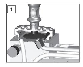
Lift diaphragm carefully sidewise. Never use a pointed or sharp-edged tool to lift the diaphragm.
