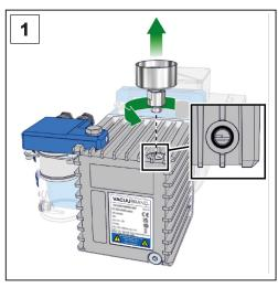
Unscrew the manometer at its adapter from the oil reservoir of the rotary vane pump; open-ended wrench width 17 mm. Do not turn the manometer itself as leaks might be caused! Pay attention to the O-ring.
