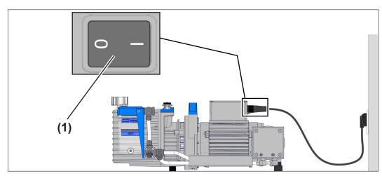
$\Rightarrow$  Switch rocker switch (1) on – switch position I.
