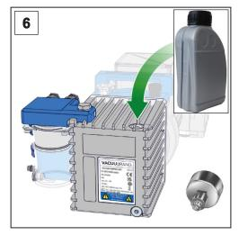
6. Add approx. 100 ml (0.11 quarts) of pump oil. Observe the oil level through the sight glass in doing so. The oil level must be between the marks "min." and "max." on the rating plate. Do not overfill.
