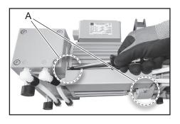
→ Remove the cover plate. Use a Phillips screw driver size 2 to loosen both screws (A). Pay attention to lock washers.
