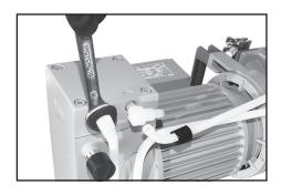
→ Slip the hoses onto the hose connectors by turning the fittings with an open-ended 14 mm wrench.
