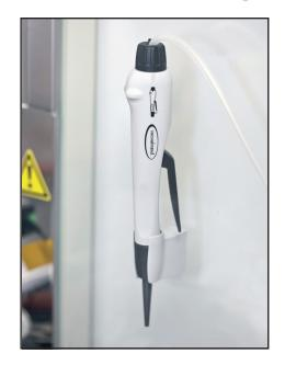
For keeping, position the VHC<sup>pro</sup> in the wall holder.
