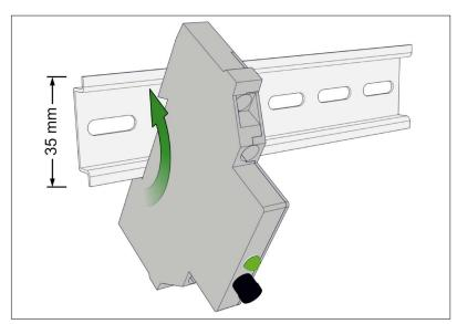
⇒ Clip the analog module onto the 35 mm hat rail, e. g., inside a switch cabinet or a distribution box.
