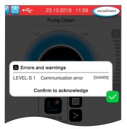
The **error indication** must be acknowledged after the error has been remedied.
