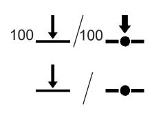
Vacuum control to a preset vacuum value (here: 100 mbar/Torr/hPa); (without / with VACUU•BUS-compatible VARIO pump)
