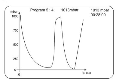
When selecting "Graphic", the display shows a pressure vs. time curve.
