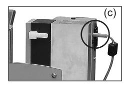
➤ Connect the VACUU•BUS cable from the CVC 3000 controller to the Peltronic emission condenser (c).
