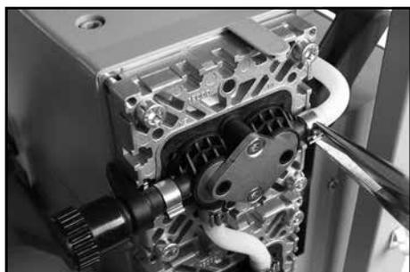
Affix the connection tube (V) to the other side of the pump at the valve head (O).
