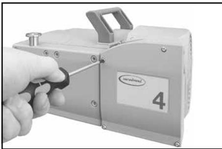
The pigtail fuses are integrated into wires ((1), black and blue) inside the terminal box. To replace the fuses it is necessary to replace both wires completely (fixed with flat pin bushings (2)).
